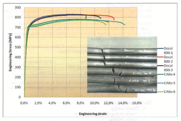
Figure 1: Tensile tests of the tubes.
