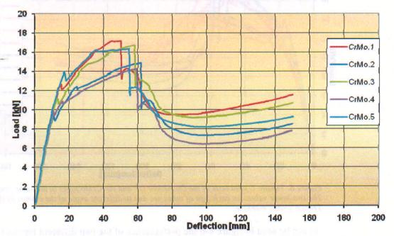
Figure 4: Tensile T-jopint tests of the 4130 CrMo tubes. The two lower values are due to different angle of the clamps in the Tensile testing machine.
