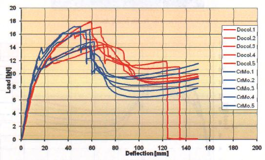
Figure 6: Tensile T-joint tests of the Docol 800 DP and the CrMo tubes in the same graph. The two lower values on each type of tubes are due to different angle of the clamps in the Tensile testing machine.
