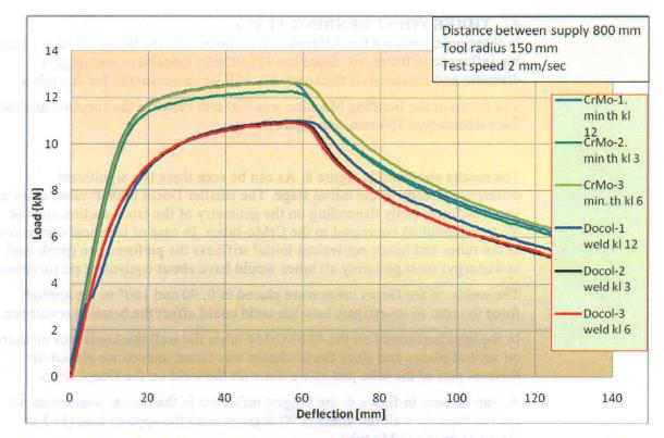
Figure 8: Three point bending test of the tubes.
