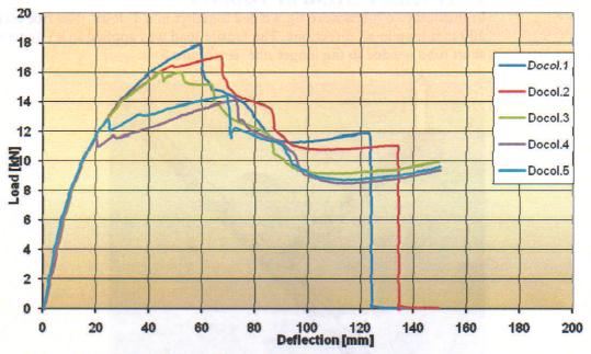
Figure 5: Tensile T-joint tests of the Docol 800 DP tubes. The two lower values are due to different angle of the clamps in the Tensile testing machine.
